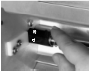
Stripper pad adjustment
