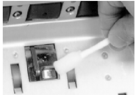
Magnetic pickup head (quantity 2) - Wipe surface using dry foam-tipped swab, also wipe tension spring. The second head is on the movable plate.
