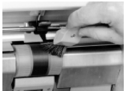
Feed wheels (quantity 2) - Brush each wheel using a side-to-side motion to remove paper dust from the grooves. Vacuum area when finished.
