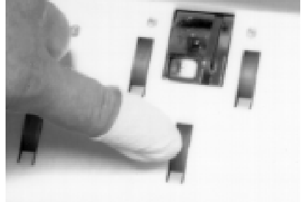
Pinch rollers (quantity 5) - Brush paper dust from areas around the rollers and wipe each using a cloth moistened with the approved professional cleaner.
